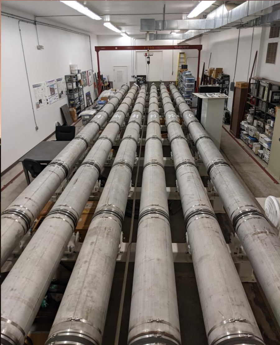
The six fast delay line vacuum tubes
