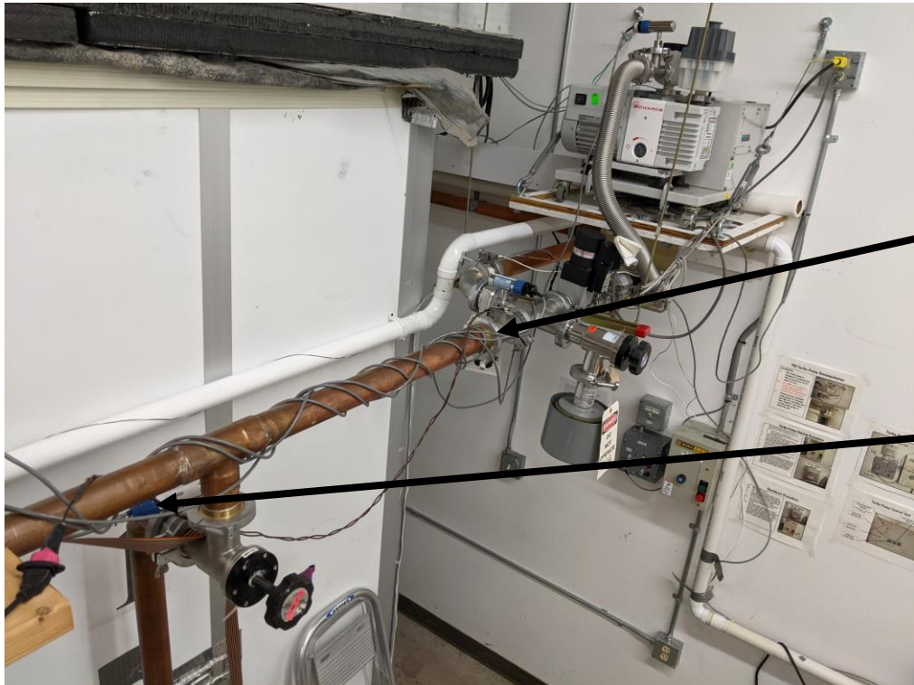
Pump and previous vacuum manifold
